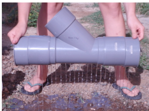
Figure 5. Rainfall simulation apparatus; 0.5 m length of PVC pipe with an opening on the top for the addition of water and 24 holes on the bottom (0.3 cm diameter each) spaced approximately 1 cm apart to dispense water on to experimental plots.
