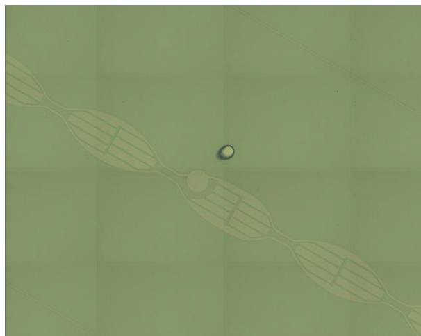
Figure 5. (A) These images of the detector were put together without flat field averaging. The seams where they were stitched together are visible because of the variation in lighting across the image. (B) Using flat fielding, these systematic variations can be removed, creating a much smoother looking image. Note: the difference in contrast is not caused by the flat fielding.
