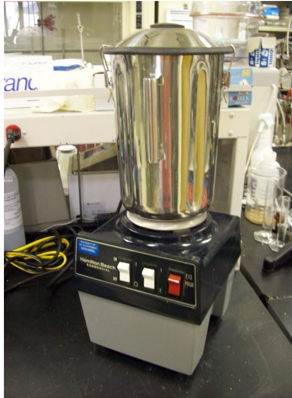
Figure 3: Industrial sized blender used to mechanically reduce the particle size of biomass samples.
