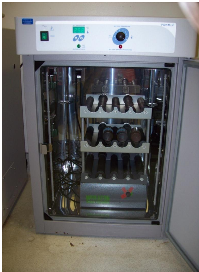
Figure 2: The roller bottle apparatus used for rotating the enzymatic hydrolysis roller bottle reactors enclosed in an incubator held at 48.5 °C.
