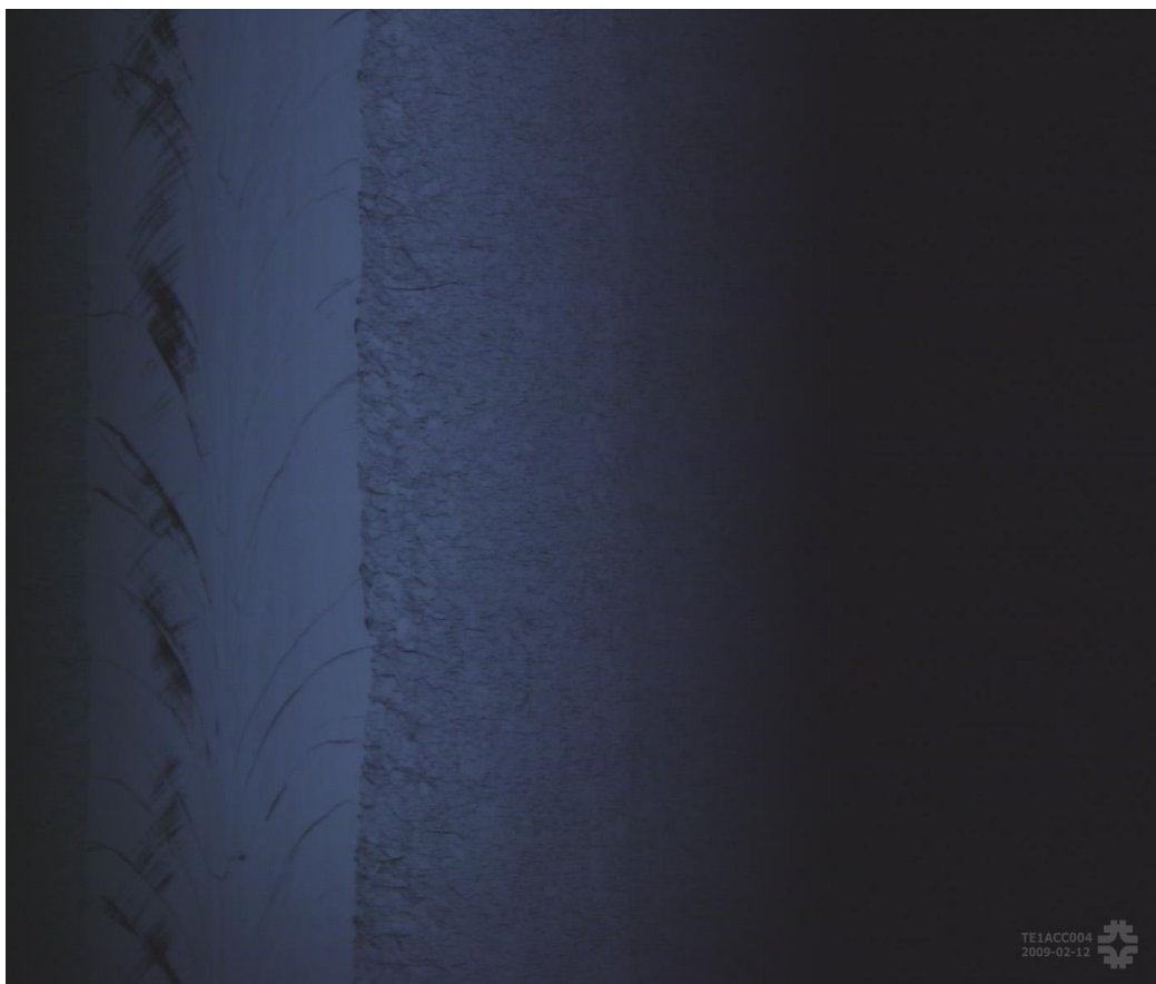
Figure 4. The weld line after initial BCP and EP, with no mechanical polishing.
