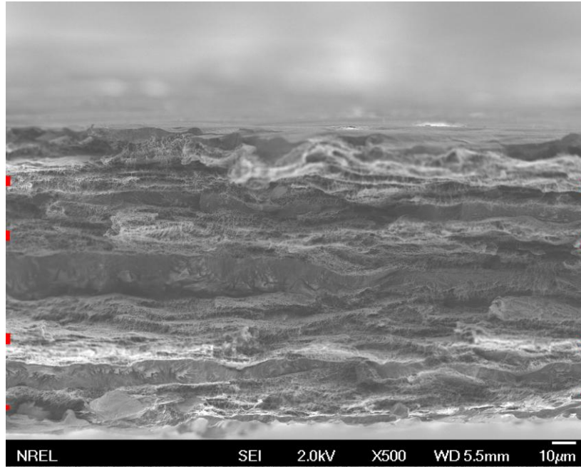
Figure 10: FE-SEM of four ply EPON 828 & Epikure 3245 sample 38 at 500x. The red dashes indicate start and end of buckypaper layers. Note the epoxy layer thickness in comparison to Figure 9.
